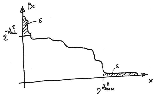
$\rightarrow$  potentially "save" lots of resources by allowing a small probability of failure. For example, by allowing a failure probability  $\varepsilon$  in data compression, we can use only  $H_{\max}^{\varepsilon}(X)$  bits.
